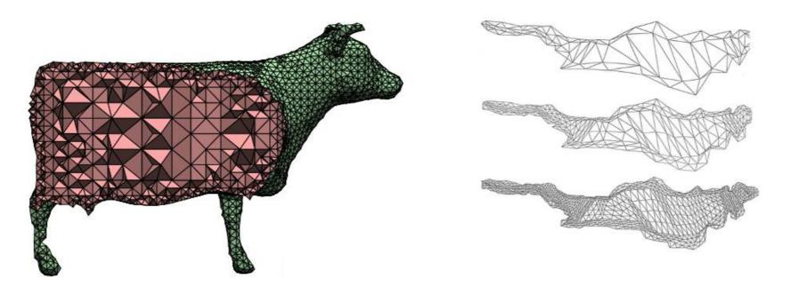
Automated 3D multigrid sequence of meshes - 2D multigrid sequence of meshes, created manually
